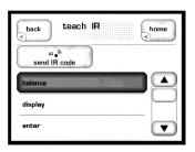
The CP-500 provides discrete infrared (IR) command codes for all its functions, a list that extends far beyond what is required by normal remote controls. However, many of these functions are critical if you plan to create a customized remote control with macros that take command of your entire system. Without these discrete codes, many of the macros you might want to create will simply not work reliably.
